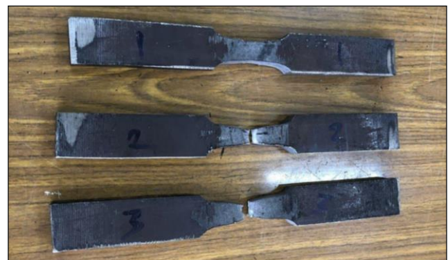
Fig. 5 Tensile test specimens after a fracture.
