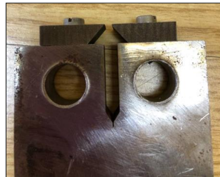
Fig. 8 Pre-cracking by WEDM.
