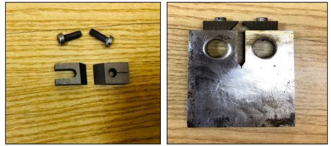
Fig. 13 Attachable knife-edge design.
