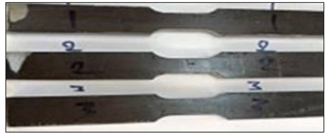
Fig. 3 Dimension tensile test specimens before fracture.
